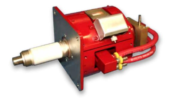
A magnetron is a high power microwave oscillator in which the potential energy of an electron cloud near the cathode is converted into RF energy in a series of cavity resonators. The VMX3095 magnetron delivers high peak and average RF power for use in medical or industrial applications.
